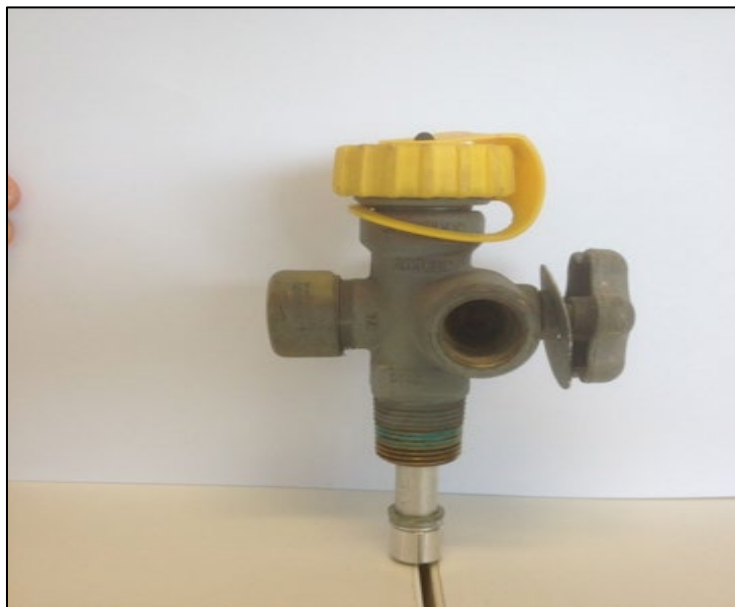
Figure 26. In-situ gas cylinder showing removable yellow cap
