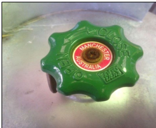
Figure 27. Exchangeable gas cylinder showing green tap with 'OPEN' and 'CLOSE' markings
